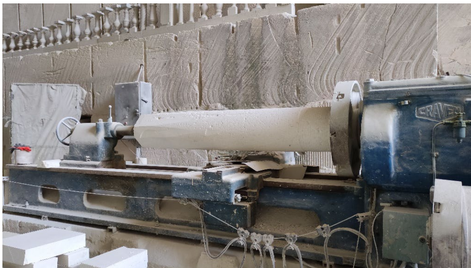
column carving on a lathe – Sarragan quarry – Les Baux de Provence
